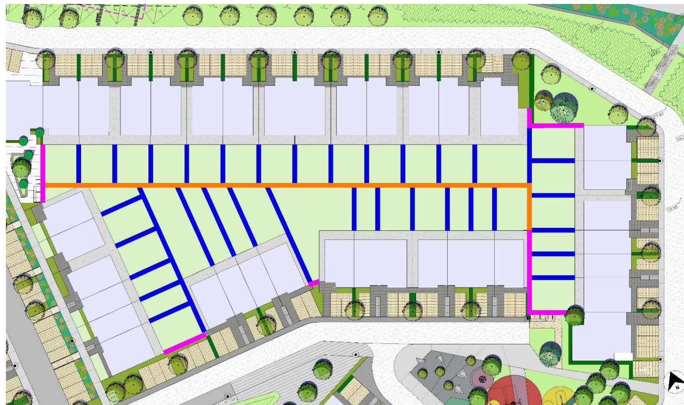
Retaining wall between rear gardens 2000mm high rendered concrete blockwork wall
